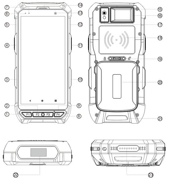
①F1 ②F2 ③Volume ④Reserved Button ⑤USB port ⑥Blue Led Indicator ⑦Red LED indicator ⑧F3 ⑨F4 ⑩Power Button ⑪Reserved Button ⑫Reserved Pogo Pin ⑬Front Camera ⑭Receiver ⑮Rear Camera ⑯Label ⑰Flashlight ⑱RFID Reading Area ⑲Battery Cover Locker ㉑Battery Cover ㉑Wrist Strap Locker ㉑Barcode Scan Window ㉑Cradle Pogo Pin Connector
